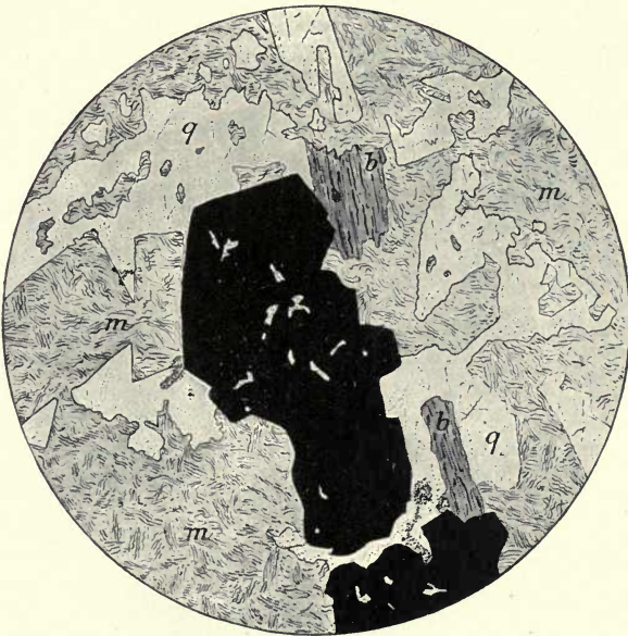
Altered Granodiorite. Bellefontain mine, Nevada City, Cal. m , Fine aggregate of sericite, with a little calcite and secondary quartz, replacing orthoclase and andesine; b , original biotite altered to sericite; q , original quartz; black, pyrite with included sericite. Magnified 15 diameters. (559)
